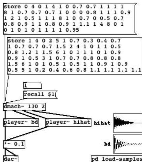
Figure 2: A `dmach~` two voice drum machine.
